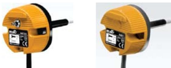
The BAE72 & BAE72-S Thermolectric tripping device operates in conjunction with a spring return actuator to drive a motorized fire damper to its "safe" position in the event of the preset maximum temperature being exceeded.
